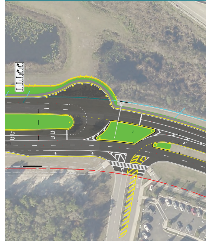
North Mid-Block U-Turn at Rinehart Rd
