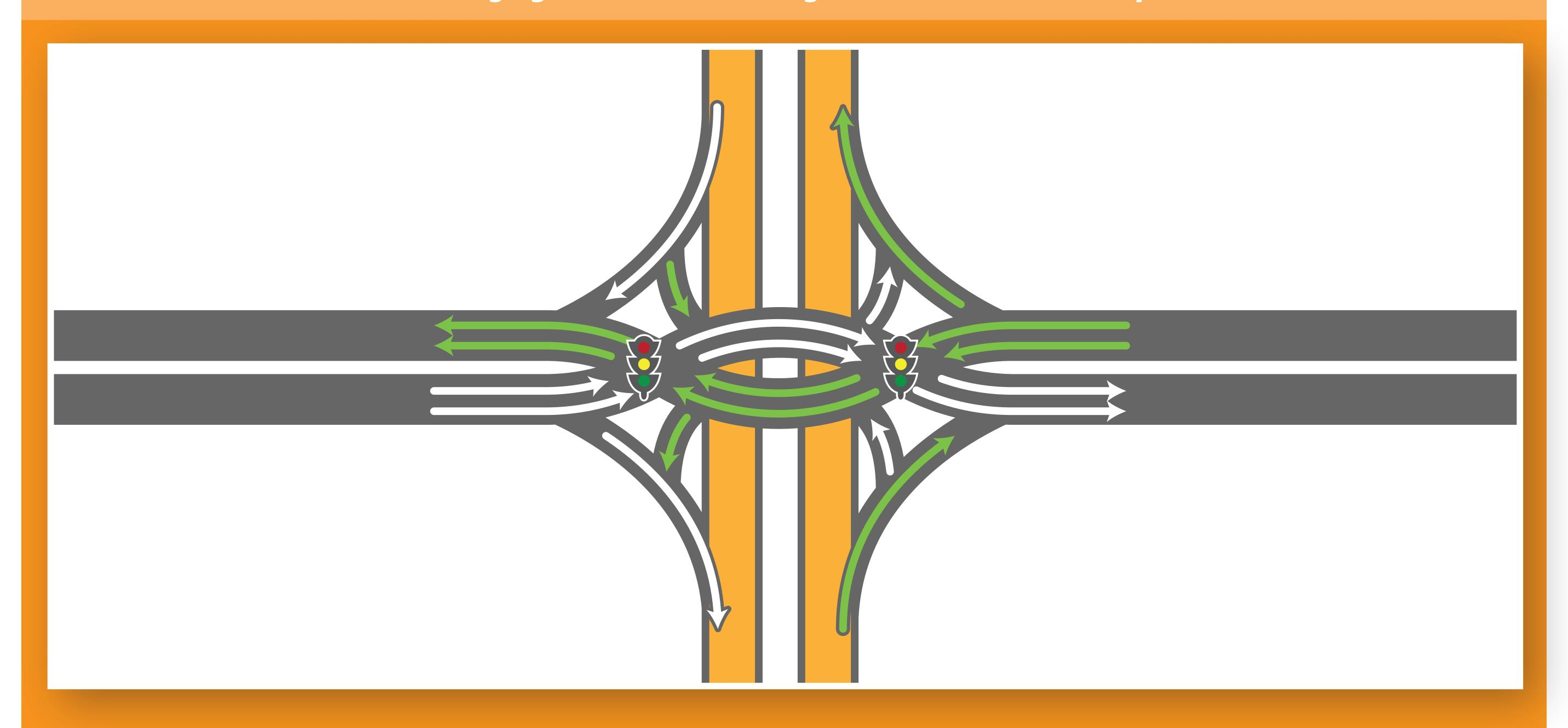
The diverging diamond interchange (DDI) eliminates left turn phases at traffic signals. It also reduces the number of traffic signal phases from four to two phases. The DDI will move almost double the traffic through the intersection in the same time.
