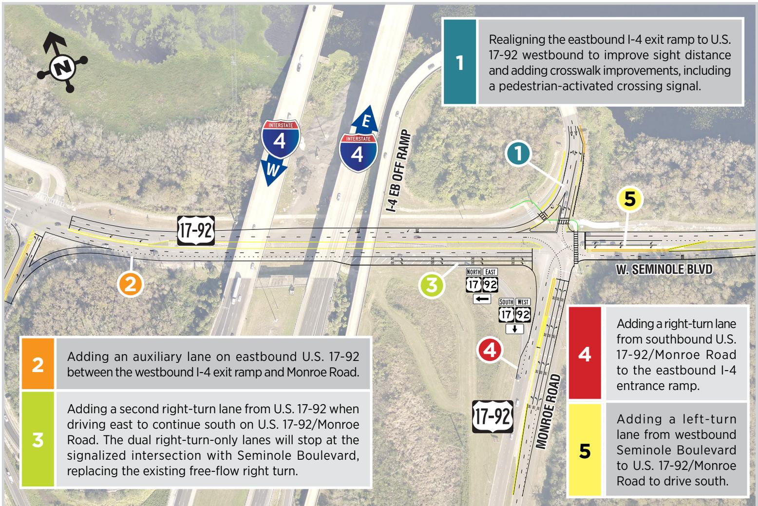
**1** Realigning the eastbound I-4 exit ramp to U.S. 17-92 westbound to improve sight distance and adding crosswalk improvements, including a pedestrian-activated crossing signal.
