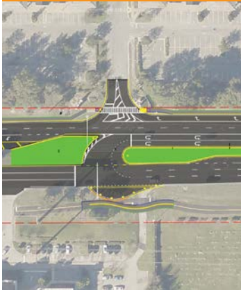
South Mid-Block U-Turn at Rinehart Rd
