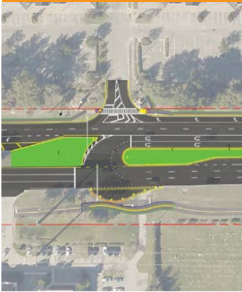
South Mid-Block U-Turn at Rinehart Rd
