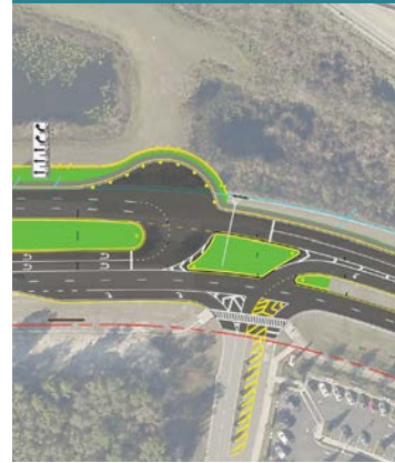
North Mid-Block U-Turn at Rinehart Rd
