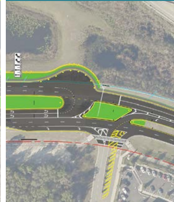
North Mid-Block U-Turn at Rinehart Rd
