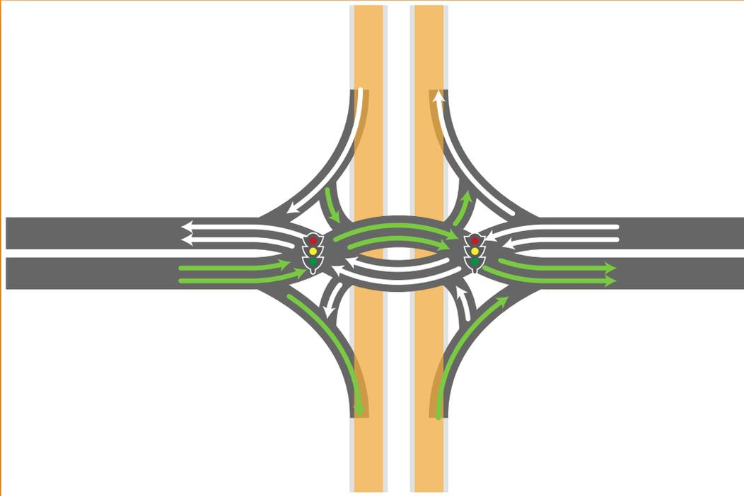
The diverging diamond interchange (DDI) eliminates left turn phases at traffic signals. It also reduces the number of traffic signal phases from four to two phases. The DDI will move almost double the traffic through the intersection in the same time.
