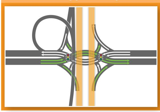
The diverging diamond interchange (DDI) eliminates left turn phases at traffic signals. It also reduces the number of traffic signal phases from four to two phases. The DDI will move almost double the traffic through the intersection in the same time.
