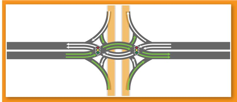
The diverging diamond interchange (DDI) eliminates left-turn phases at traffic signals. It also reduces the number of traffic signal phases from four to two. The DDI will move almost double the traffic through the intersection in the same time.
