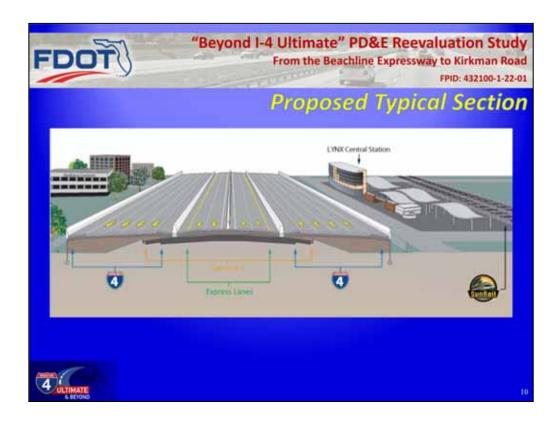
The proposed typical section for the I-4 improvements is shown here. The typical section consists of four express lanes in the middle, three general use lanes on either side and one auxiliary lane between interchanges.
