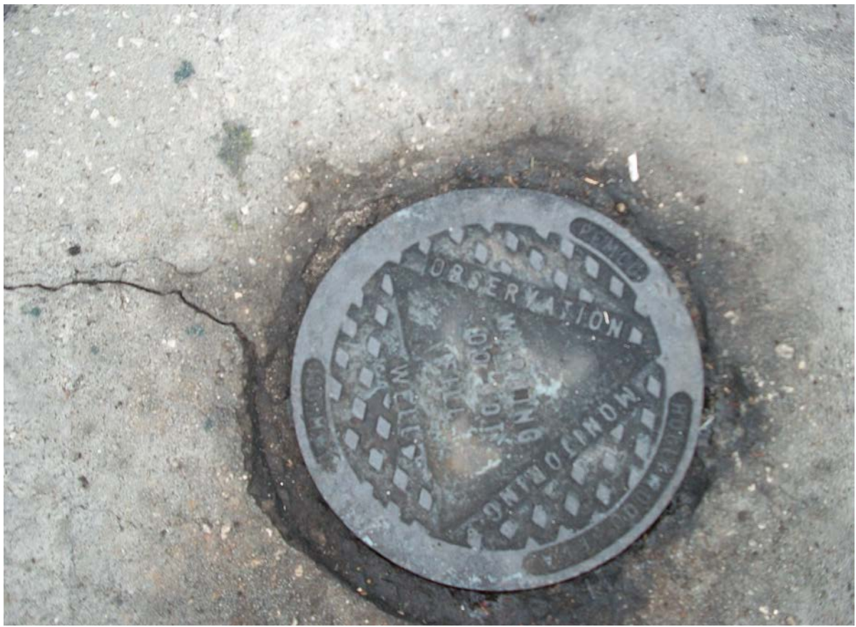
Site 66: Checkers Restaurant (former Chevron #42157) – monitoring well east of Checkers building in the parking lot
