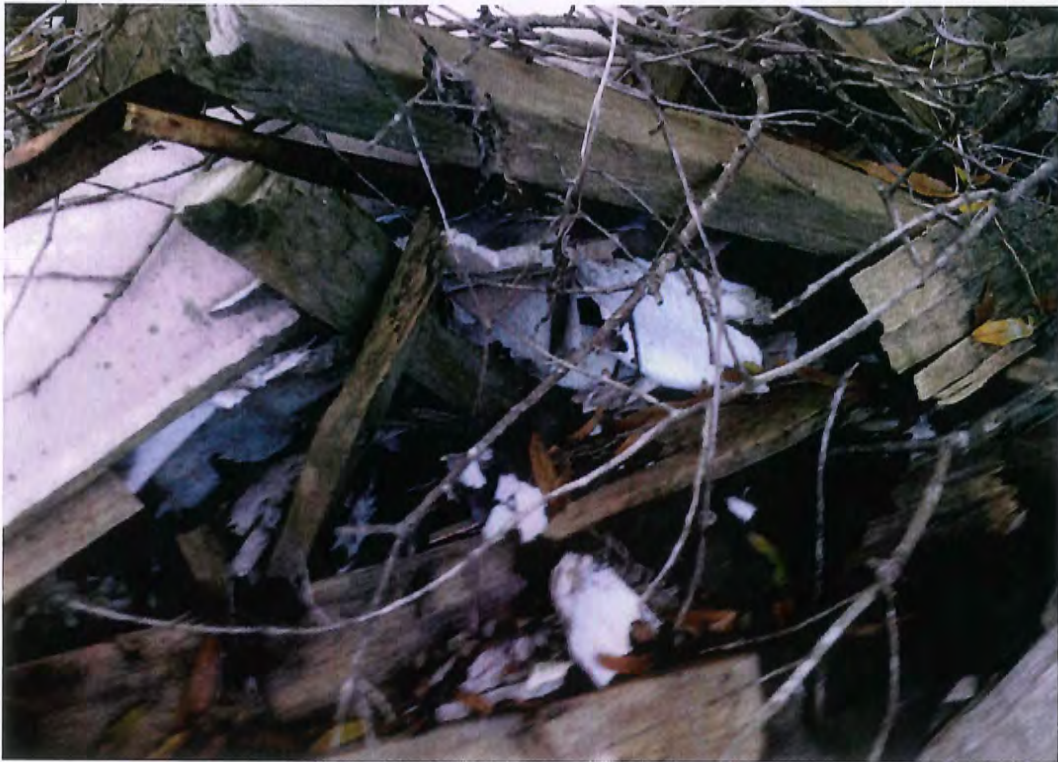
19. View of homogeneous area BDP1-4, gypsum wall board, located in Building Debris Pile #1. No asbestos was detected in homogeneous area BDP1-4.
